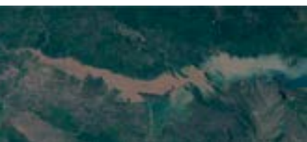
Above: Figure 2: Highly turbid waters entering the Cahora Bassa reservoir in Mozambique, indicating sedimentation issues. (c/ EOMAP contains Copernicus data from 2020)
